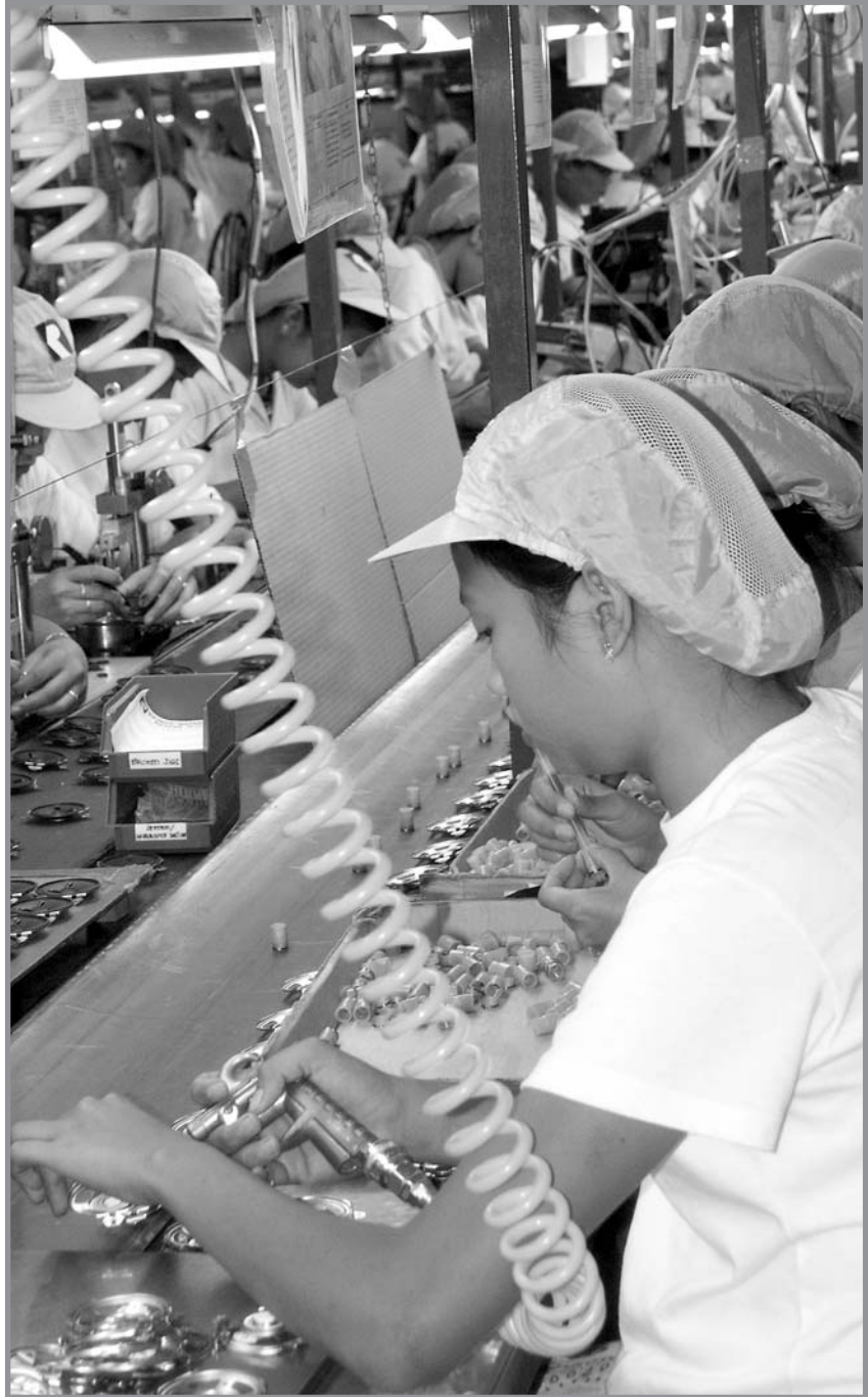
Sticking job in the production line for acoustic components for telephones and computers at the Keyrin factory in Cavite.
